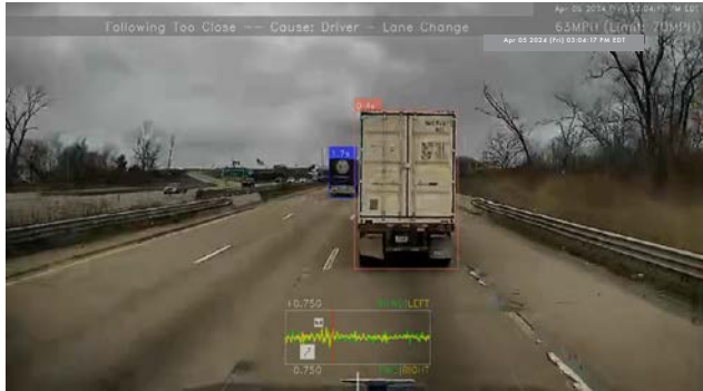
In-cab systems capture video, speed, traffic conditions, hard braking, upcoming traffic signals, and various other metrics, which allow for feedback and improvement for drivers.
